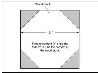
Figure 17. Cross-section of turning stock.
